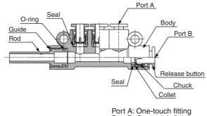
Port A: One-touch fitting Port B: One-touch fitting Stud
